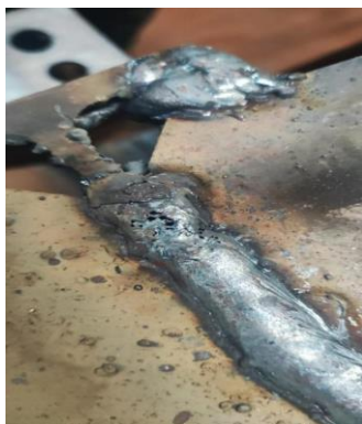
Gambar 6. Gambar Jenis Cacat Poros Cluster
